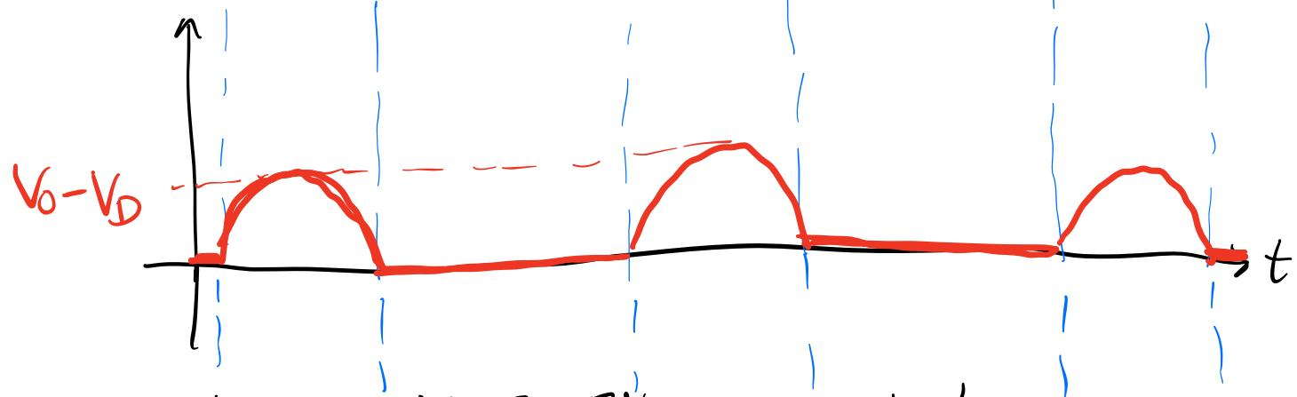
When  $V_{in} < V_D \approx 0.7V$ , no current  $\Rightarrow V_{out} = 0$ .
